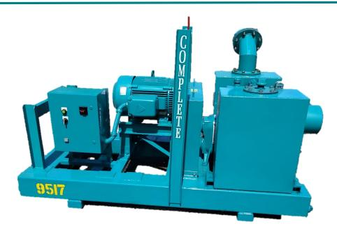
protect pump end components during periods of dry run and reduce surges in discharge and header lines. And since the rotary lobe pump end handles both the air and water together, there is less maintenance required than with priming assisted pumps. A piggy-back V-belt drive system reliably transfers power to the industry leading all cast iron Vogelsang wet-end. Optional motor mounted gear drive system available.
